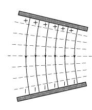
Tip: (i) Note that  $E = -\Delta v / \Delta x$  is smaller at the bottom than at the top.
