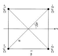
By symmetry, the electric field must be along the y-direction.
